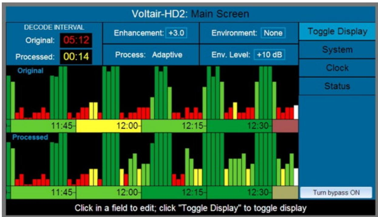
There are parallel confidence displays: "Original" represents watermarking confidence for the encoder alone. "Enhanced" represents watermarking confidence after adaptive enhancement processing by Voltair. If Enhancement is set to 0, there is no enhancement processing applied and these graphs will be identical.
